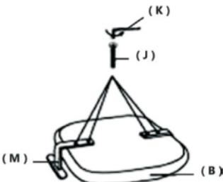
**3. Fasten the backrest A to the seat B mountings. Do this on both sides of the backrest A. Use the screws J and hex wrench K.**
