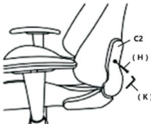
**5. Fasten the butterfly mechanism over the seat B. Use the screws J and hex wrench K.**
