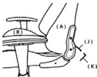
**4. Fasten the side protective covers C1 and C2 over the seat B mountings. Do this on both sides of the backrest. Use the screws H and hex wrench K.**
