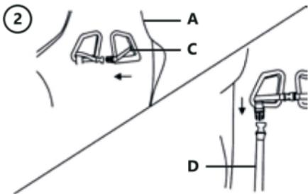
**7. Place the chair face down and insert the star base into the butterfly mechanism D**
